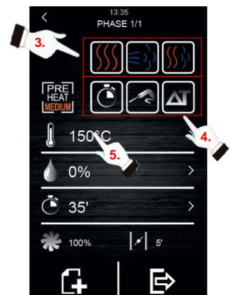
• **Selecting the temperature set point of the cooking cooking chamber (only possible with time-controlled cooking mode and core probe):**
