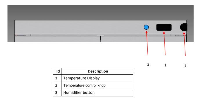
There is one variable that the user can regulate, which is temperature. This is affected by the type of food and the quantity introduced into the fermenter. The temperature is regulated with the knob shown, in a range of 85°C. To turn the equipment on, press the knob once.
