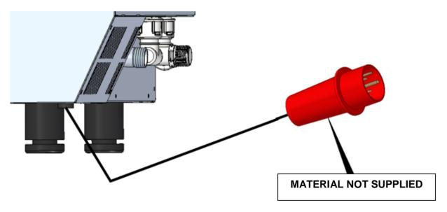
In order to prevent damages from unintentional reset of the cutting thermal device, this unit should not be fed by an external control device, such as a timer, or be connected to a circuit whose supply is regularly interrupted.
