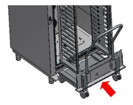
Ensure the correct movement of the trolley inside the oven, avoiding blows or obstructions that can cause the leakage of liquids and lead to possible burns.
