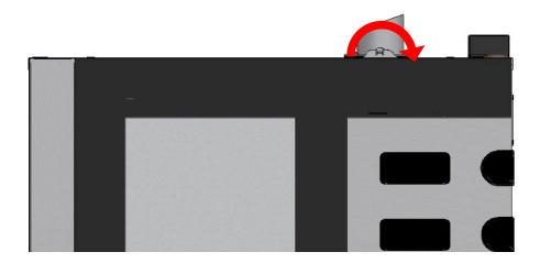
Burn Hazard: Before changing the chimney draft, verify that the oven is cold. If not, you should use thermal mittens or similar to avoid possible burns.
