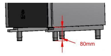
Check the length of the diagonals of the oven inlet, and they must be identical. If not, act again on the regulation of the legs.
