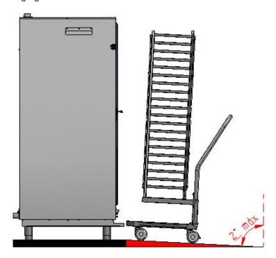
In case of exceeding the maximum angle of entry of the trolley into the oven, there is the possibility of spills of hot liquids that can lead to burns.
