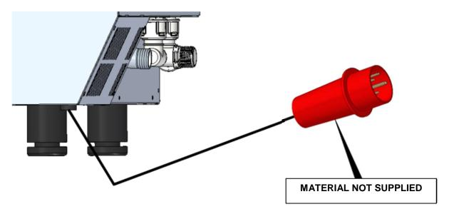
In order to avoid any danger due to accidental rearmament of the thermal cutting device, this device must not be powered by an external control device, such as a timer, or connected to a circuit whose power is interrupted regularly.
